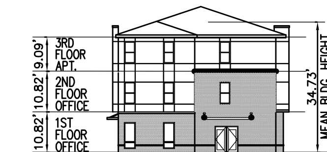
COMMERCIAL OFFICE / APARTMENTS FRONT ELEVATION
